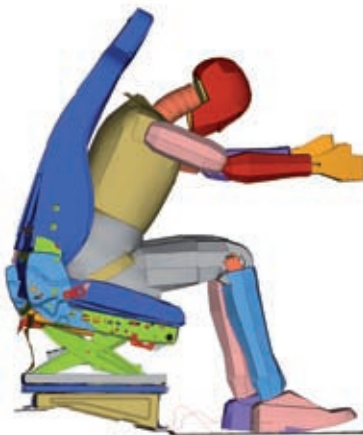
Figure 3: Crash test on sled – comparison of simulation results (left) and real test results (top)
