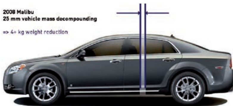
Figure 3: Reducing the vehicle length of a Chevrolet Malibu (2008) about 25 mm saves 4 kg in weight
