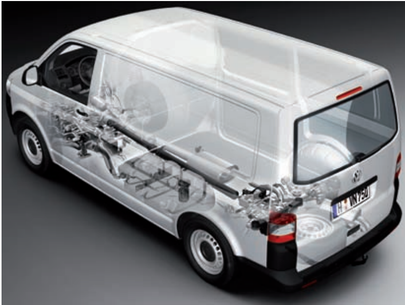
Figure 5: T5 Transporter „4Motion“ with 132 kW engine and DSG
