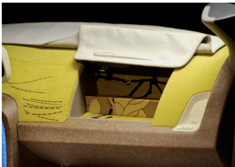
Figure 4: Foldable glove compartment: the fabric slides away easily
