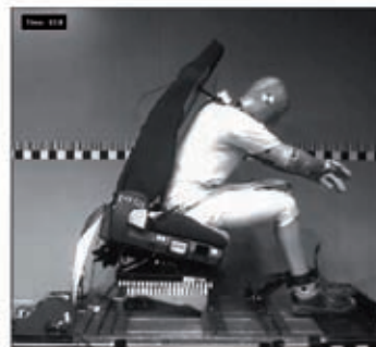
Figure 3: Crash test on sled – comparison of simulation results (left) and real test results (top)
